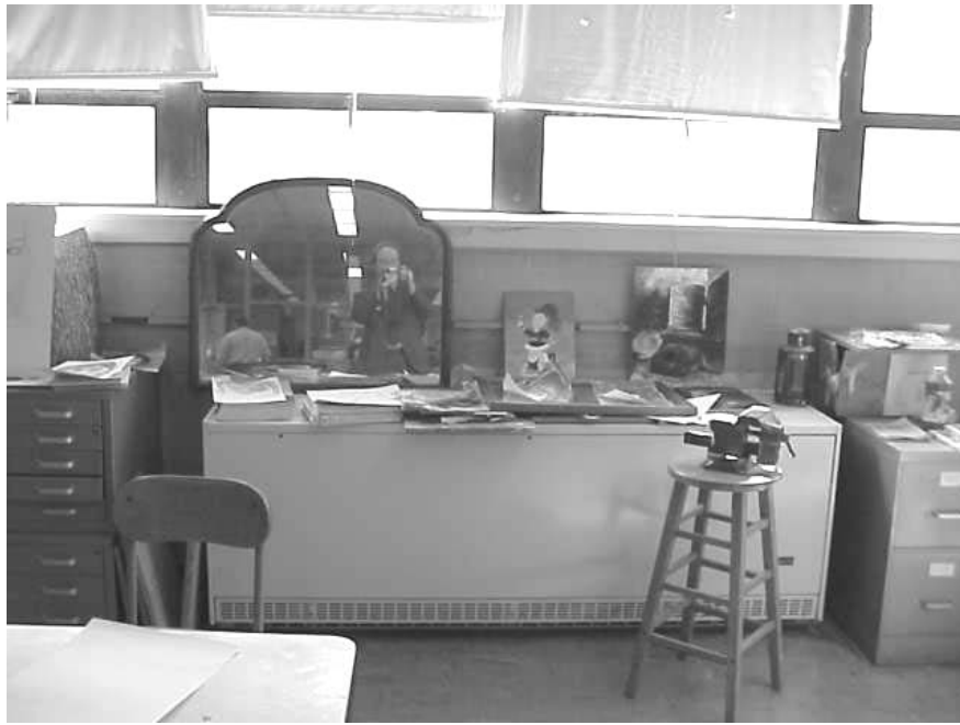
Materials Stored on Univent Obstructing Univent Air Diffuser
