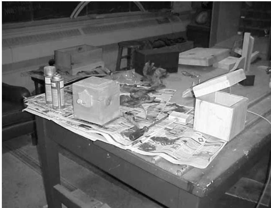
Spray Painted Materials with No Local Exhaust Ventilation
