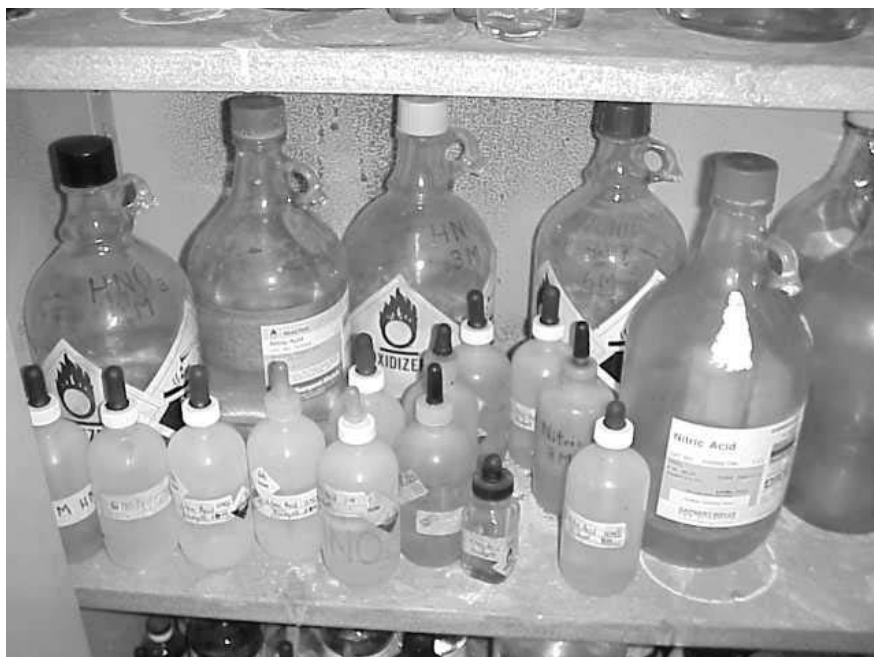
Acids Stored In Steel Flameproof Cabinet, Note Corrosion of Shelves and Cabinet Walls
